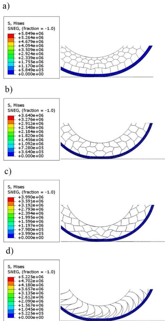
Figure 4. deformed shape of spoke structures and local stress in spokes [pa] under a vertical load of 4000 N: a) hexagonal honeycomb with 48 units, b) NPT-A1, c) NPT-C1, d) Spoke pair model
