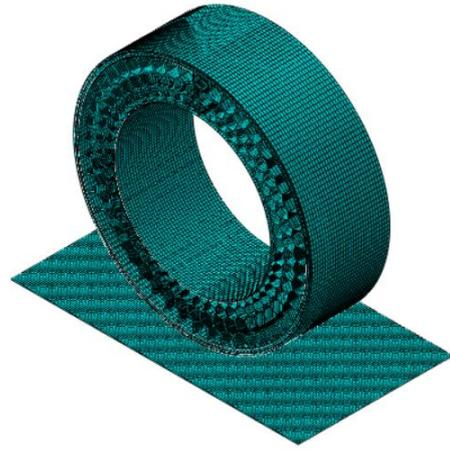
Figure 2. Meshed hexagonal NPT model with 48 units
